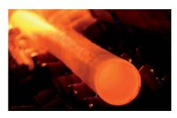
As a result, these fine-grain structural steel grades are characterised by maximal yield strength rate, good weldability and high resistance to brittle cracking. These grades are used mainly for hydraulic engineering, heavy machinery, shipbuilding and crane constructions.
